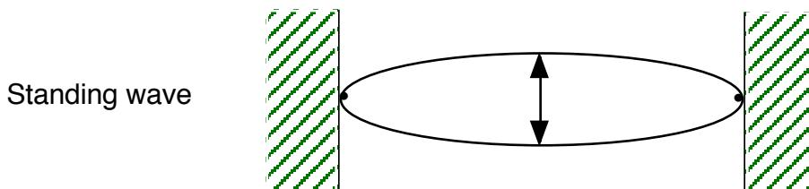
Any element of a standing wave executes SHM corresponding to a velocity of  $(F/\mu)^{1/2}$ , even though the wave does not appear to move along the string. Because the wave velocity may not be apparent, it is sometimes more intuitive to think in terms of  $f$  and  $\lambda$  [frequency and wavelength].
