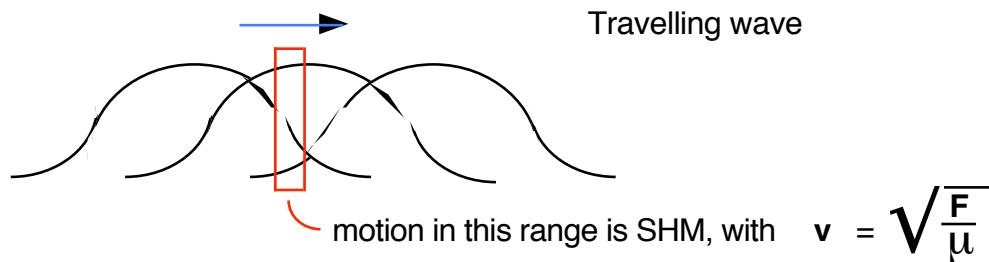
Now, if the string is fixed at each end, then there is no motion at the end points, and the wave is called a *standing wave*:
