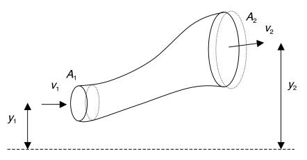
At end #1, the total mechanical energy of the volume element is  $E_1 = 1/2 \Delta m_1 v_1^2 + \Delta m_1 g y_1$
