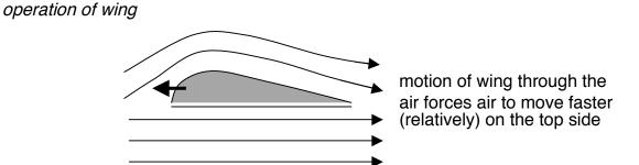
pressure is lower on the top side of the wing because the air is moving faster ---> pressure difference gives the wing lift
