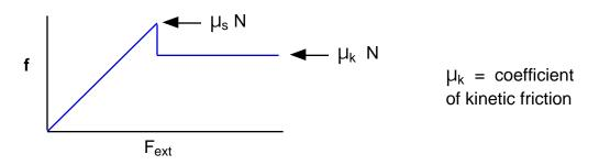
In the class demo, the coefficients of friction are found for aluminum on wet wood:
