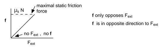
The maximum force of static friction,  $\mathbf{f}_{max}$ , is
