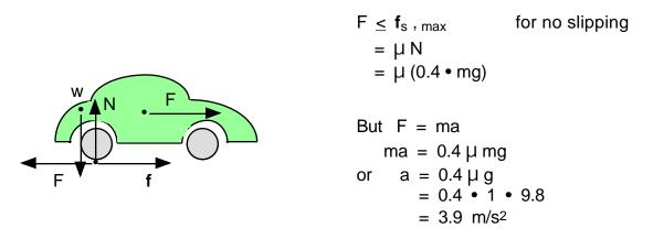
How long would it take for this car to go from 0 to 100 km/hr = 28 m/s? From  $\mathbf{v} = \mathbf{at}$ , then  $\mathbf{t} = 28 / 3.9 = 7$  seconds. Theoretically, if all of the weight were over the drive wheels, then  $\mathbf{a} = 9.8 \text{ m/s}^2$  and the time for 0 to 100 km/hr would decrease to 28 / 9.8 = 3 seconds.
