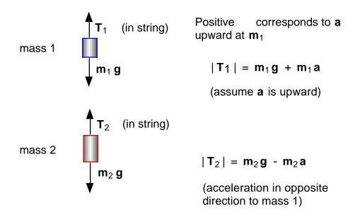
If there the string slides over the pulley without causing it to accelerate, the tension is constant along the string and the two equations can be solved to give **a**:
