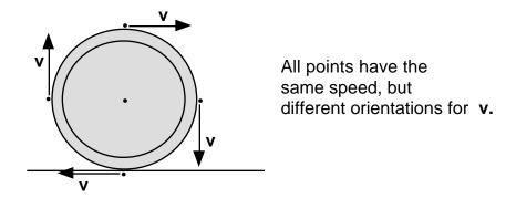
According to an observer stationary with respect to the ground, add  ${\bf v}$  to each velocity above:
