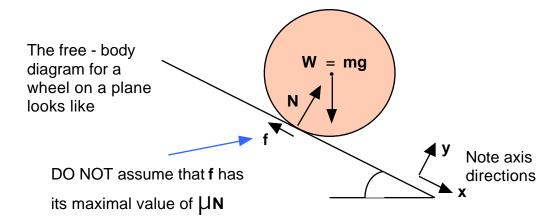
The effect of the frictional force is to produce a torque about the axle.
