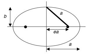
The semi-major and semi-minor axes a and b are indicated on the diagram. By definition, the sum of the distances from a point on the ellipse to the two foci is 2a, so the heavy line in the diagram must have a length a (by symmetry). Whence, by Pythagoras:
