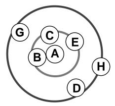
We can define a region, indicated by the outer circle, beyond which NO particle could have reached A within the elapsed number of trial moves. If the number of moves is small, then the outer circle is small; clearly the size of the circle grows with time.
