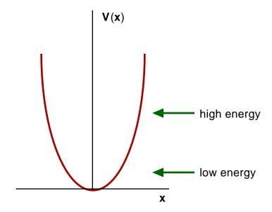
At high total energy (kinetic plus potential), the particle can move through a modest range of x, while at low total energy, its range is more restricted. At zero energy, the particle occupies a unique ground state at x = 0. If this particle is placed in thermal contact with a large system at a fixed temperature, then we would find:
