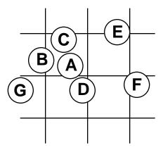
The straight lines indicate the fixed boundaries of the neighborhoods. The advantage to the fixed neighborhoods is that it is an order N operation to assign all the particles to boxes, rather than the  $N^2$  evaluation of distances required to assign particles to moving neighborhoods. The disadvantage to the technique is the overhead required to update the lists of particles in each box, and the memory taken up by the fixed array.
