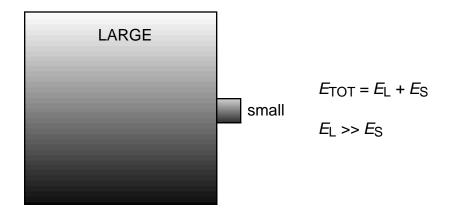
Consider now the situation where the total energy of the two systems is fixed at some value  $E_0$ ; that is, we now specify  $E_{TOT}$  at some numerical value, say  $E_{TOT} = E_0 = 10^6$  Joules. We are interested in a particular state r of the small system. This state has energy  $E_{\rm r}$ ,
