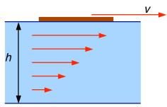
If the material in the figure were a solid, it would resist this stress until it attained a deformed configuration where the applied and reaction forces were in equilibrium. But a fluid doesn't resist shear, and the floating plate continues to move at a speed v as long as the stress is applied:
