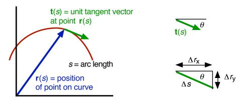
• unit tangent vector **t** has components  $(\Delta r_x/\Delta s, \Delta r_y/\Delta s, \Delta r_z/\Delta s) = (\partial r_x/\partial s, \partial r_y/\partial s, \partial r_z/\partial s)$ in the infinitesimal limit. Hence
