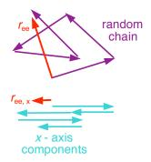
$$\mathcal{P}(r_{\text{ee,x}}) = (2\pi\sigma^2)^{-1/2} \exp(-r_{\text{ee,x}}^2/2\sigma^2)$$
