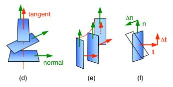
Panel (d): a series of rectangles as their orientation twists around a straight-line path. The unit tangent vector  $\mathbf{t}$  to the *path* remains fixed, so  $\Delta \mathbf{t} = 0$ . But the unit vector  $\mathbf{n}$  normal to the path and attached to the rectangle rotates around the axis of the path, so  $\Delta \mathbf{n} \neq 0$ . In panel (d), both  $\mathbf{n}$  and  $\Delta \mathbf{n}$  are perpendicular to  $\mathbf{t}$ .
