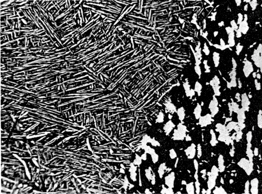
Fig. 6.19. Micrograph showing the fine basket weave structure produced in laser surface melting IMI550 (28) ( P = 1.6\text{kW} ; V = 200\text{mm/s} ; D = 0.5\text{mm} ). X 100
