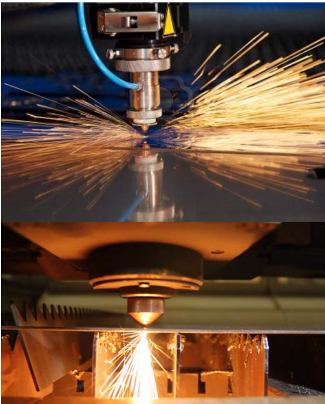
Fig. 3.22. A High Pressure Ring Nozzle used for "Clean Cut" Technique (27).
