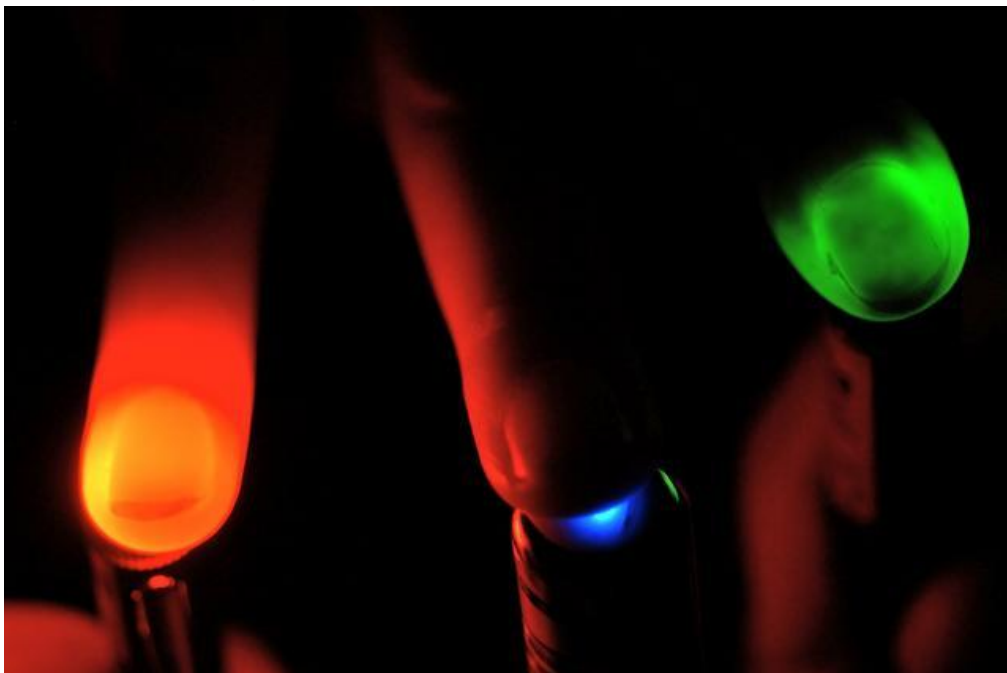
Figure 7.1 Comparative depth of penetration of laser energy in human tissue for various lasers. (Courtesy of R. James Rockwell.)
