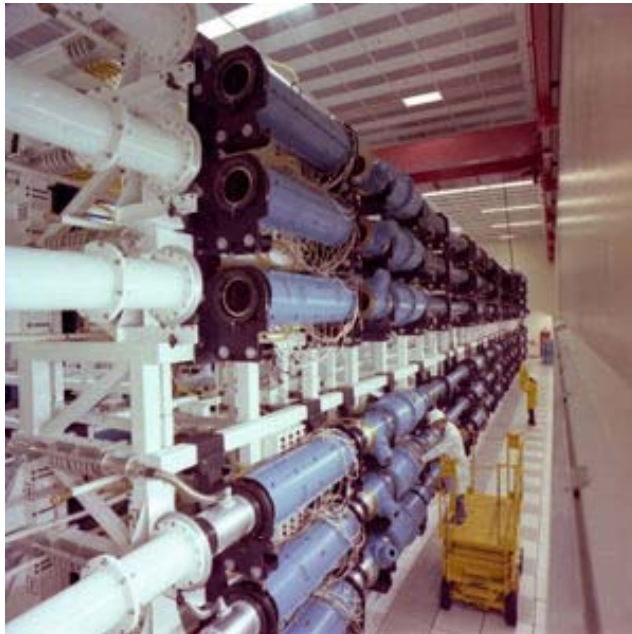
Fig. 9.12 Model of a 12-arm Shiva laser facility. The master oscillator is centrally located in the background of the figure. Each line corresponds to an Nd:glass amplifier chain. In the foreground is the combustion chamber with incoming beams arranged symmetrically about the center. The actual system contains 20 amplifier arms. (Courtesy of Lawrence Livermore Radiation Laboratory, University of California.)
