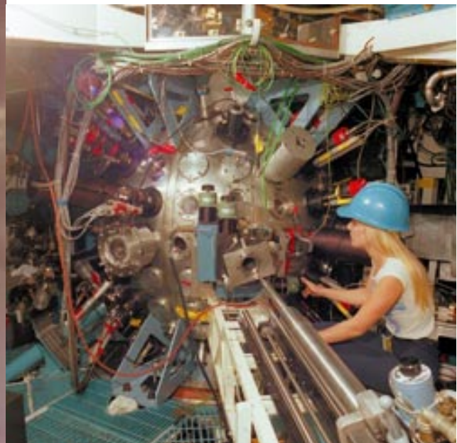
Fig. 9.12 Model of a 12-arm Shiva laser facility. The master oscillator is centrally located in the background of the figure. Each line corresponds to an Nd:glass amplifier chain. In the foreground is the combustion chamber with incoming beams arranged symmetrically about the center. The actual system contains 20 amplifier arms. (Courtesy of Lawrence Livermore Radiation Laboratory, University of California.)
