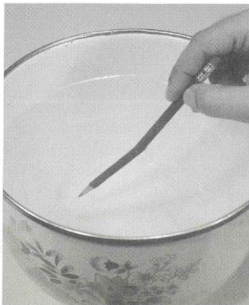
Rays from the submerged portion of the pencil bend on leaving the water as they rise toward the viewer. (Photo by E.H.)
