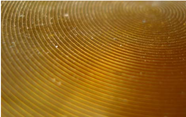
Figure 2.8 Metamorphosis of a succession of prismlets into a Fresnel lens
