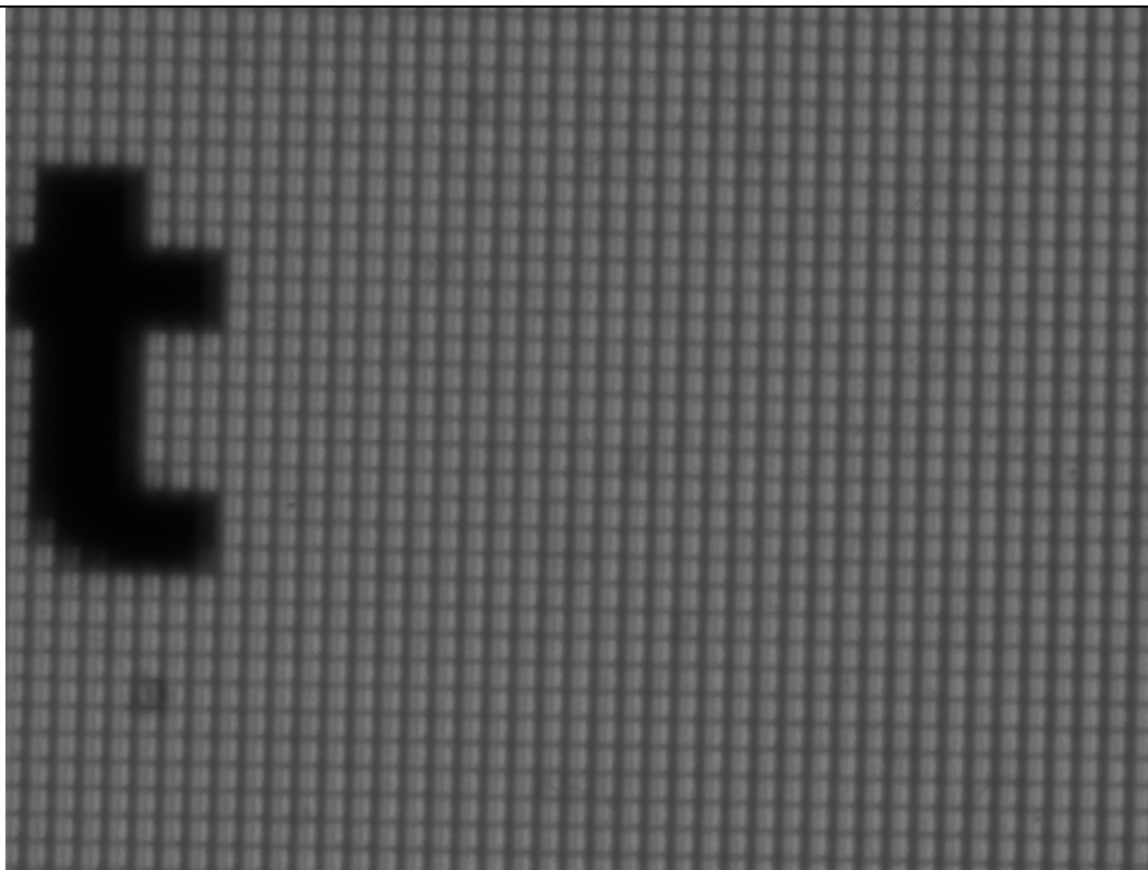
Figure 5: Captured image from LCD screen with the single lens. Dot pitch is 0264 mm on LCD
