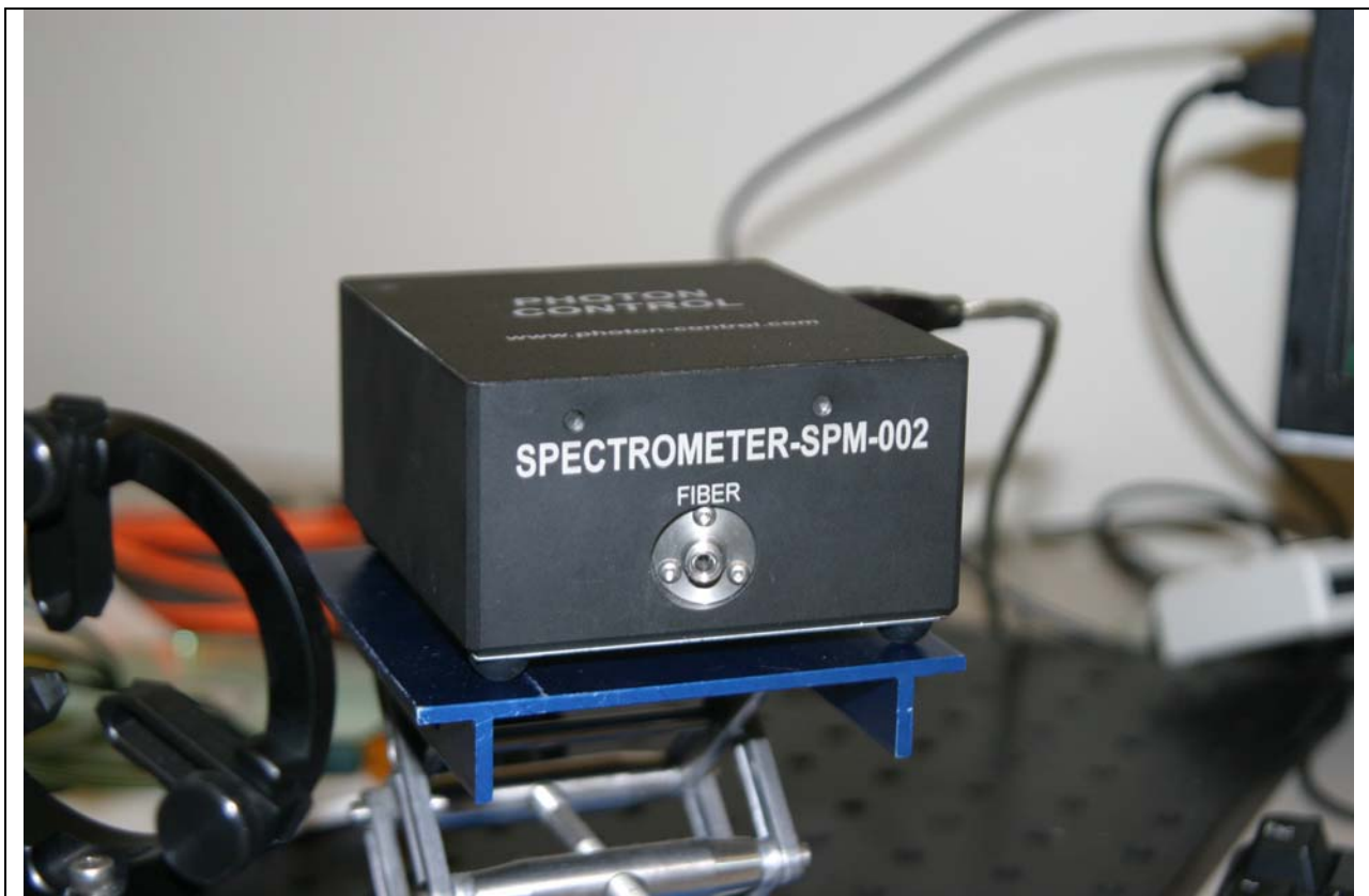
Fig. 1: SPM-002 spectrometer – note optical input port at the front
