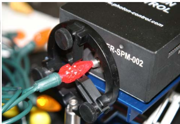
Fig. 9 closeup showing LED at optical port
