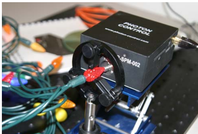
Fig. 8: LED source in mount
