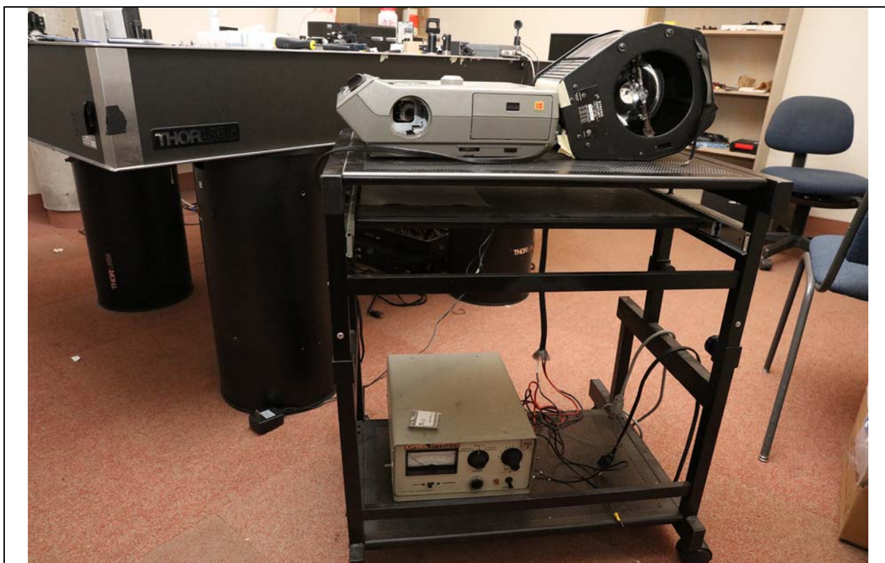
Figure 4: Table with quartz halogen slide projector (left) and mercury vapour (right) with power supply below
