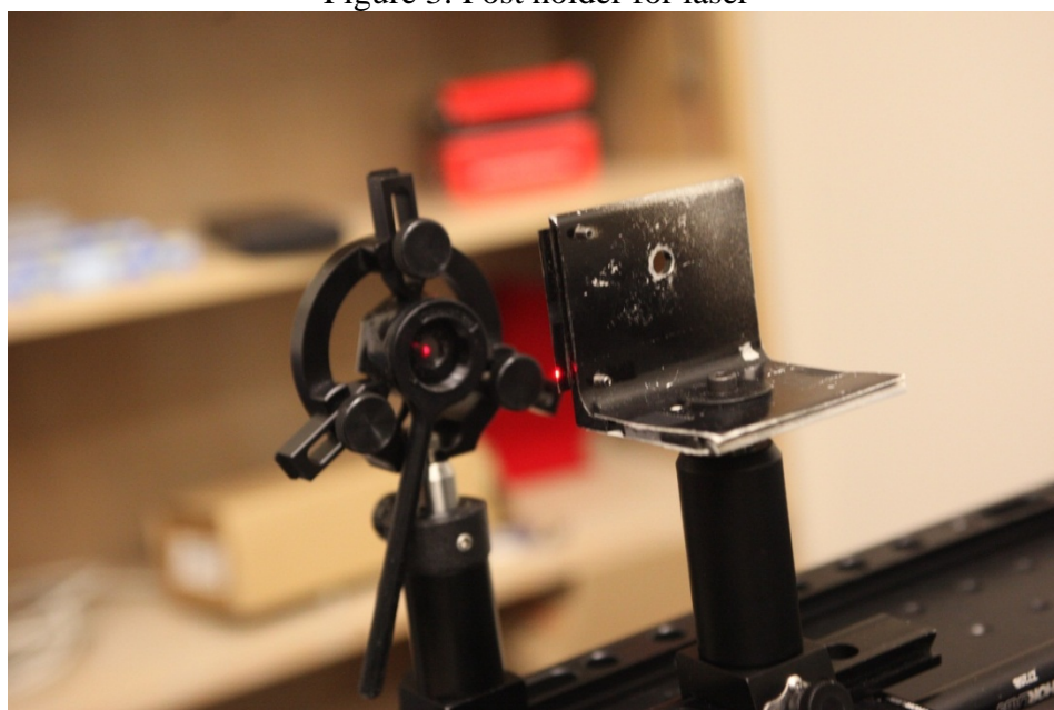
Figure 4: Silicon Detector (left) and knife edge on y axis motor (right)
