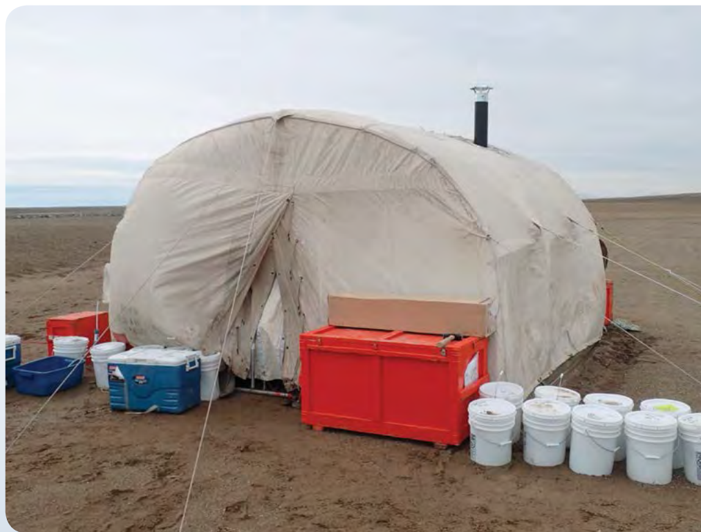
A longhouse tent and sample pails are part of a field camp at Johnson Point on Banks Island, Northwest Territories. The pails contain stream sediment and till samples that are used to recover kimberlite (diamond) indicator minerals as part of a regional provenance study.
