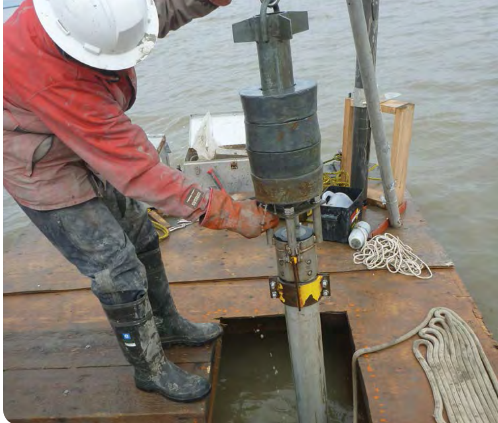
A marine sediment core is collected from Kugmallit Bay, near Tuktoyaktuk, Northwest Territories.
