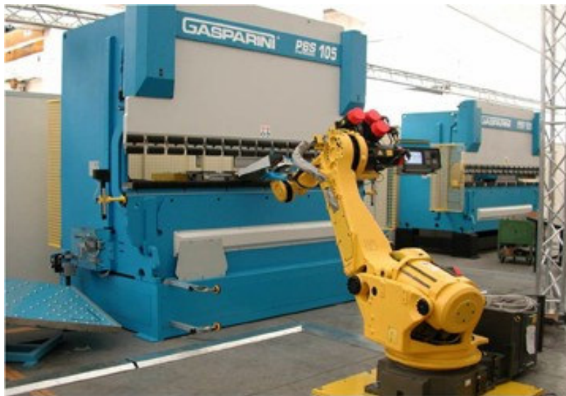
Fig 2 A robot-assisted sheet metal bending system [2] .
