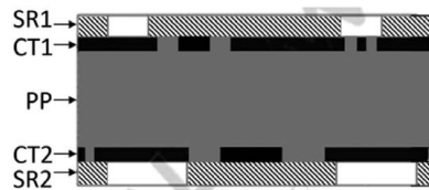
Fig. 13 Substrate cross section [50]
