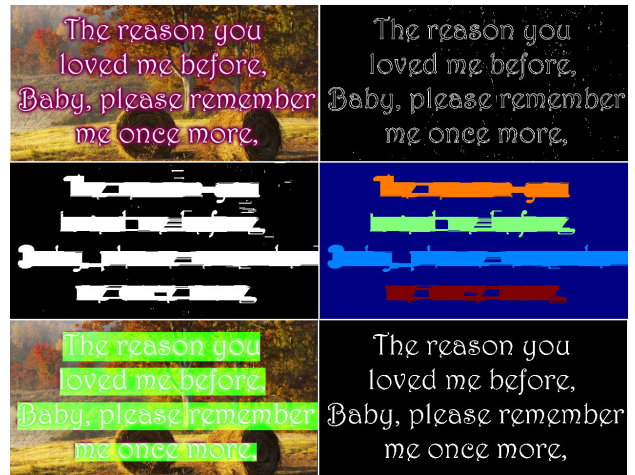
Fig. 4. An example of text detection and extraction. Top row: original image (left), edge map (right); Middle row: extended edge map (left), candidate blobs (right); Bottom row: detected text regions (left), OCR-ready binary image (right).
