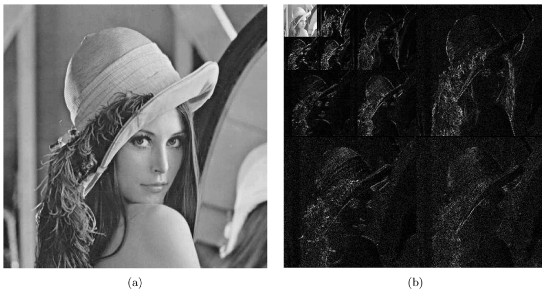
Fig. 1. Illustration of various within-subband and cross-subband correlations within the wavelet transformed coefficients. (a) Original 512 \times 512 Lena image. (b) Wavelet transformed coefficients after three levels of wavelet decomposition using 9/7 filters [14].
