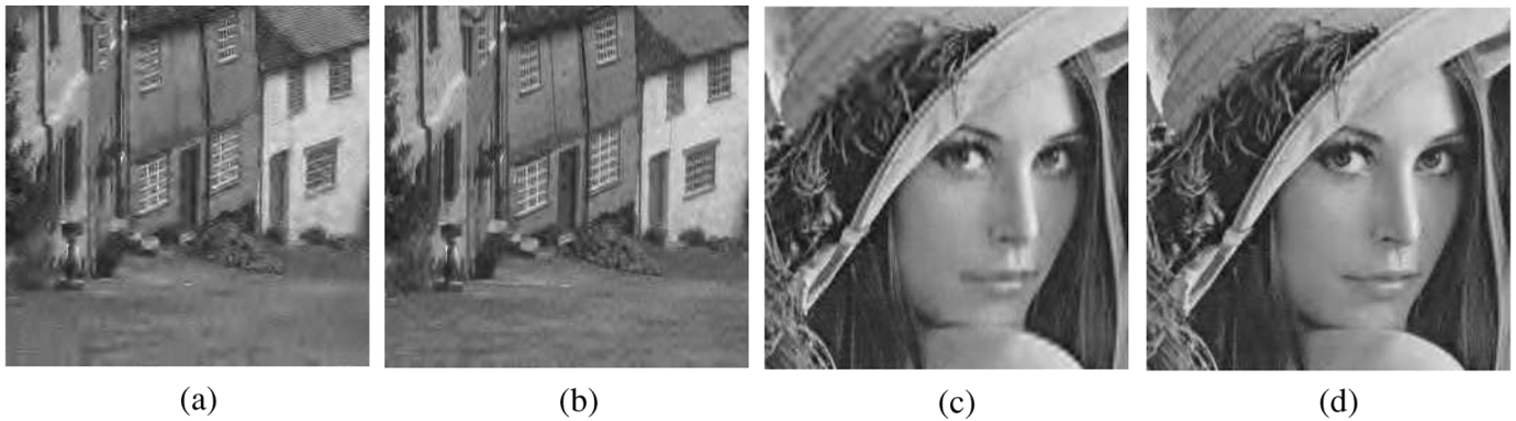
Fig. 9. Results of one side PSNR D_1 with R = 0.5 bpp per description. The other side PSNR D_2 and the central PSNR D_0 are listed in the parentheses. (a) Goldhill by RD-MDC: 30.25 dB ( D_2 = 31.00 dB, D_0 = 35.78 dB); (b) Goldhill by PC-MDFB: 31.26 dB ( D_2 = 30.81 dB, D_0 = 35.77 dB); (c) Lena by RD-MDC: 33.15 dB ( D_2 = 33.17 dB, D_0 = 39.49 dB); (d) Lena by PC-MDFB: 34.12 dB ( D_2 = 34.36 dB, D_0 = 39.49 dB).
