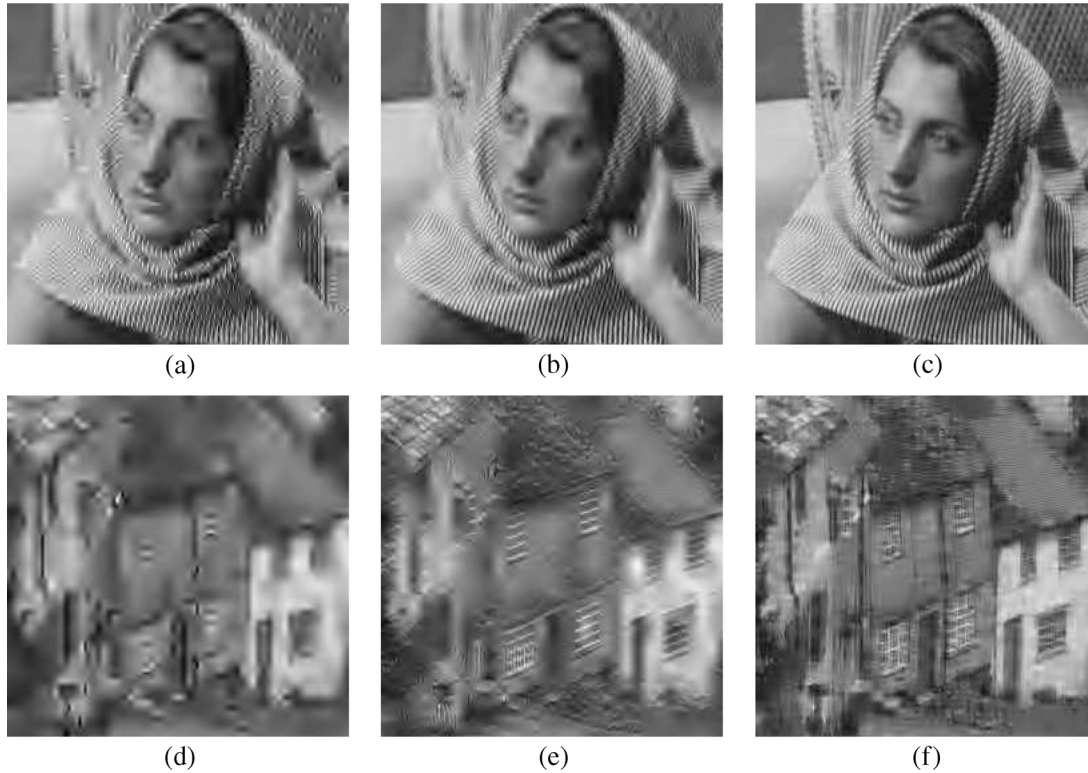
Fig. 6. Side decoder results with total rate of 1 bpp in (a)–(c) and 0.25 bpp in (d)–(f). The central PSNR is included in the parentheses. (a) Barbara by MMDSQ: 24.52 dB (36.09 dB). (b) Barbara by RD-MDC: 27.60 dB (36.07 dB). (c) Barbara by MDLT-PC: 31.68 dB (36.07 dB). (d) Goldhill by MMDSQ: 24.58 dB (30.35 dB). (e) Goldhill by RD-MDC: 24.46 dB (30.35 dB). (f) Goldhill by MDLT-PC: 27.22 dB (30.35 dB).
