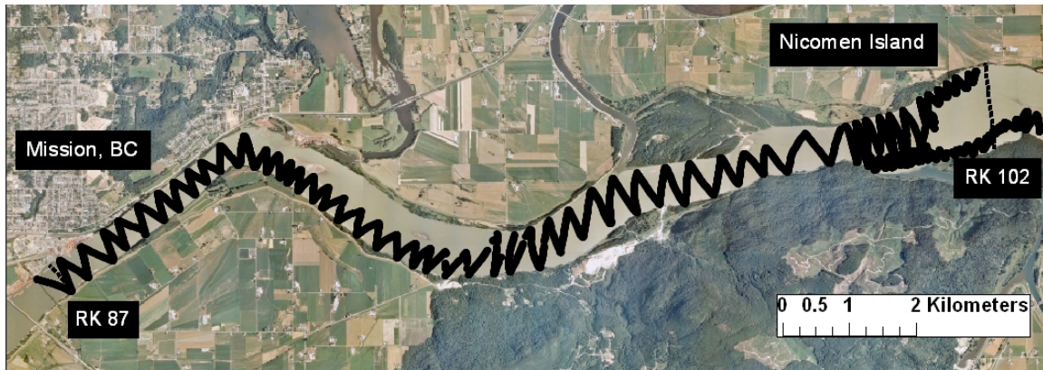
Figure 17: The “zig-zag” pattern used for field campaign 1 (April 8 th 2009 – April 11 th 2009) ADCP data collection.
