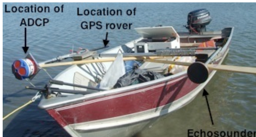
Figure 15: Aluminium boat, which deployed ADCP, GPS rover, and echosounder.
