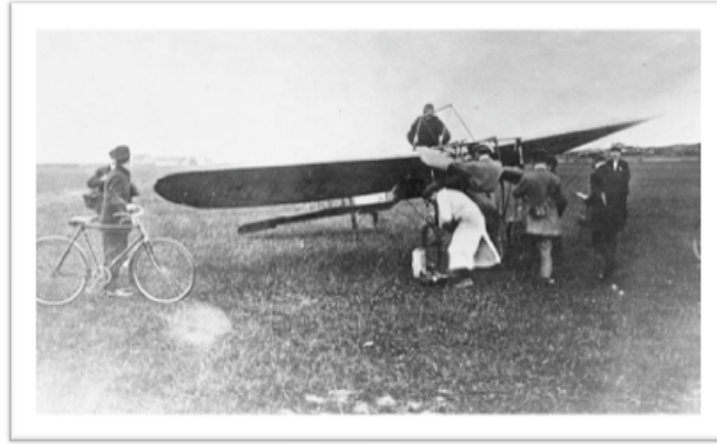
Figure 7: The Bleriot XI, the prototype for all small, single-engine propeller-driven airplanes
