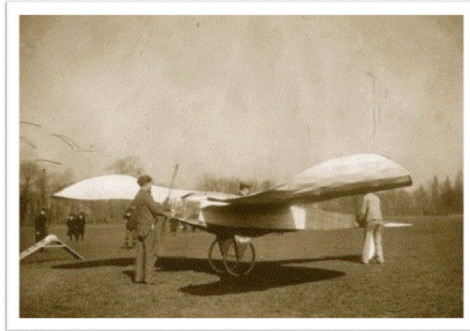
Figure 5: The Bleriot V, a bird-like pusher monoplane with forward elevator and rudder
