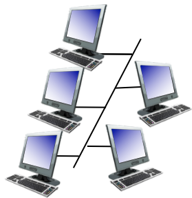
shared wire (e.g., cabled Ethernet)
