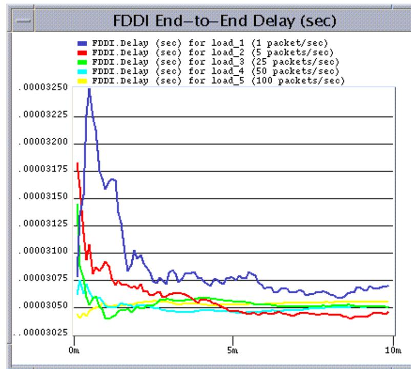
End-to-end delay (sec) plots, with load parameter (mean number of packets sent by the source) varying from 1 to 100 packets per second. Delay levels off with time, which indicates that the network is stable.
