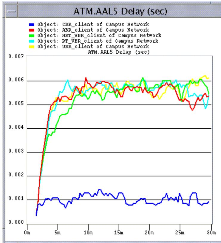
Propagation delay (sec) is the smallest for the CBR source, which has the best QoS.
