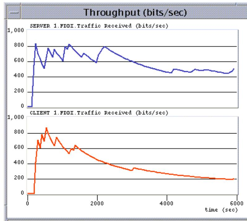
Throughput (bits/sec) plots of Server 1 (top) and Client 1 (bottom). Once stabilized, server's throughput is twice as large as the client's throughput, which is to be expected because the number of servers is smaller than the number of served clients.
