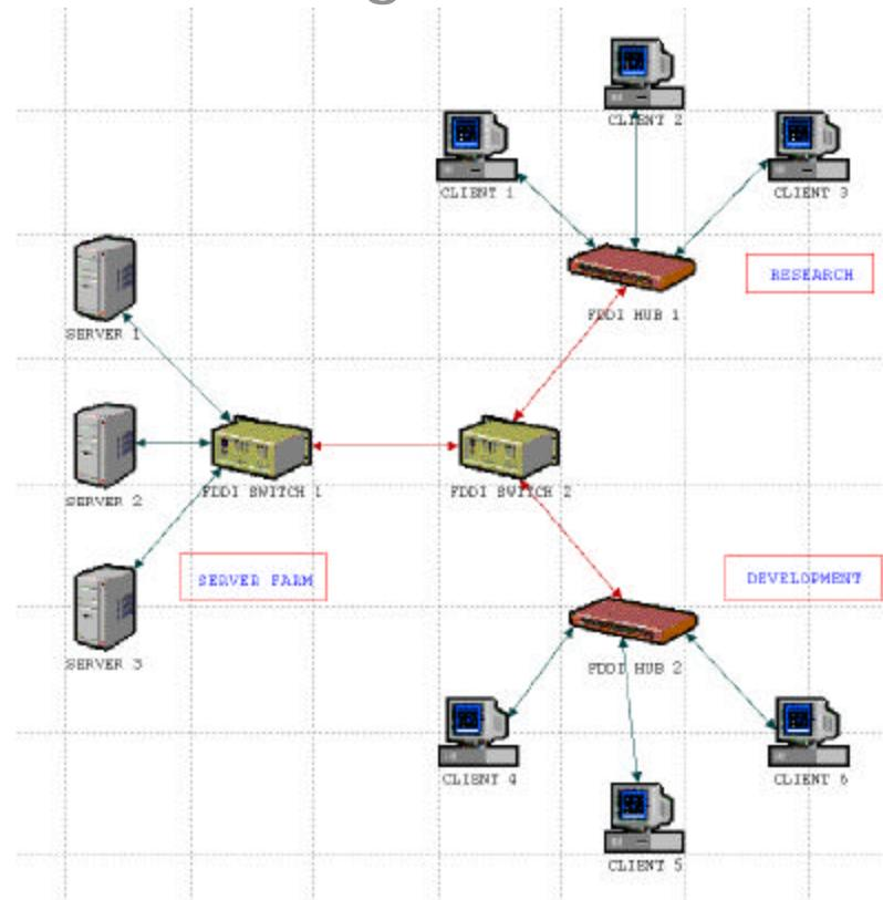
Clients are connected to the network via hubs. Hubs and servers at different locations are connected via two FDDI switches.
