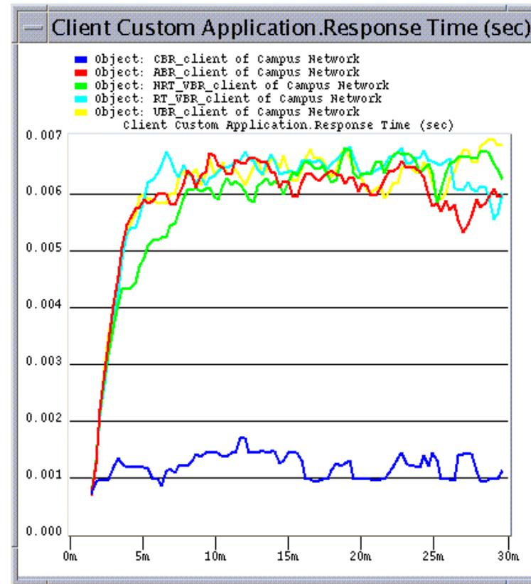
Response time (sec) for each client is the time it takes from sending a request to the server and receiving a response from it. The CBR client has the smallest response time and hence the best QoS.
