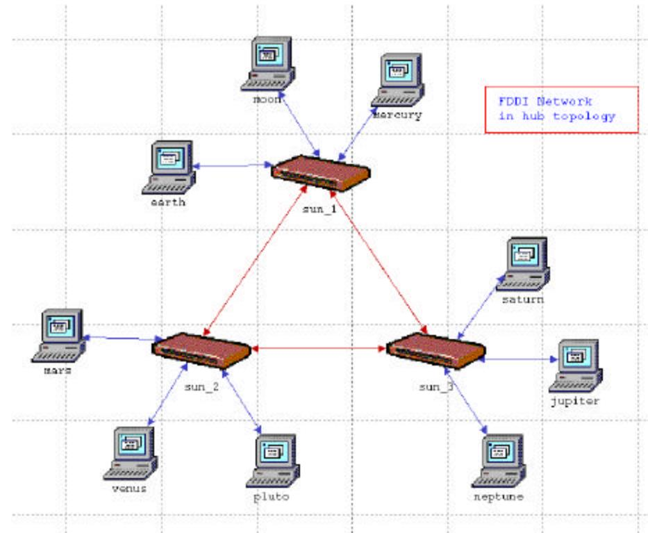
Network consists of 3 concentrators (connected with FDDI duplex links) and 9 stations (connected to the ring via concentrators).
