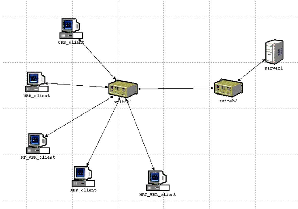
Network consists of two switches, an ATM server, and five clients requesting five distinct service categories. Traffic received by CBR client has a constant bit rate, while all other clients receive bursty traffic.
