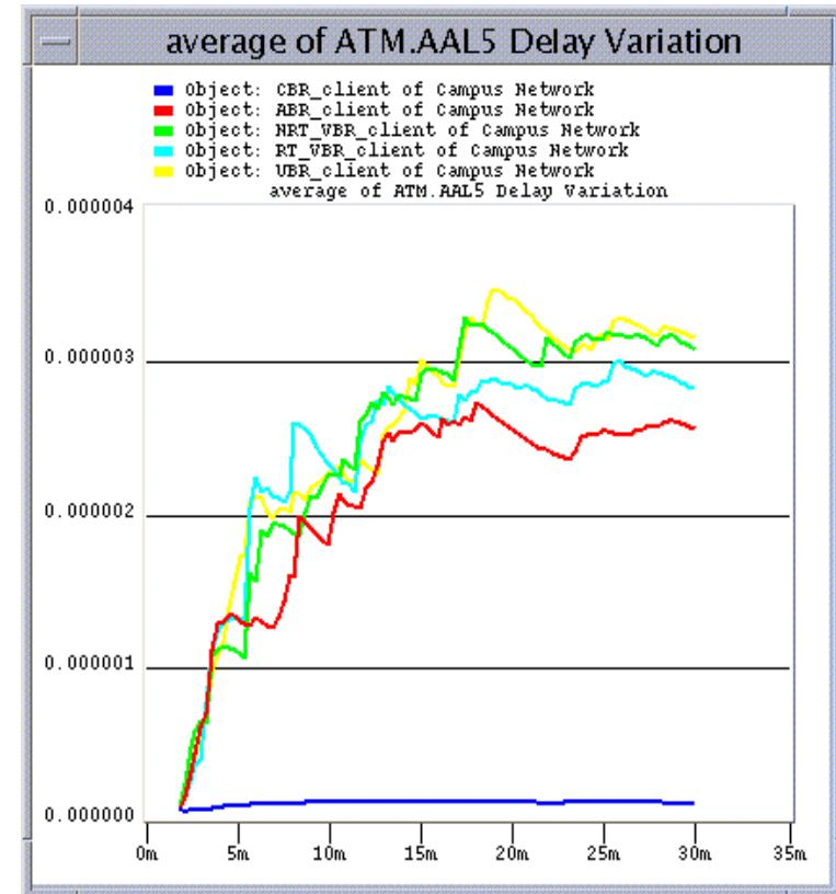
Average delay jitter is almost zero for the CBR source, which has the best QoS.
