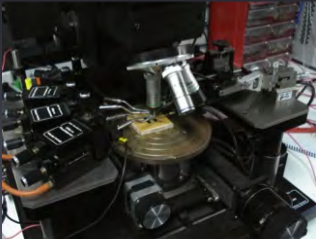
Electrical testing of RFID 915MHz (CEITEC Design)
