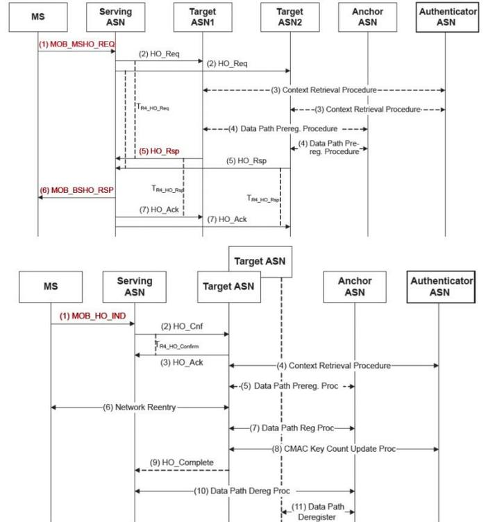
Figure 3. Flow chart of MS-initiated handover: preparation phase (top) and action phase (bottom) [7].
