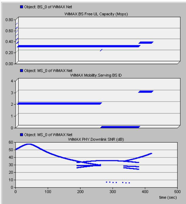
Figure 12. BS\_0 free upload capacity (top), serving BS ID for MS\_0 (middle), and downlink SNRs for MS\_0 (bottom).
