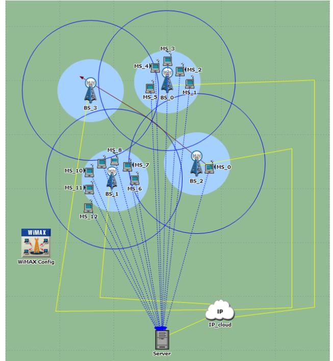
Figure 9. OPNET network model: Simulation Scenario C.
