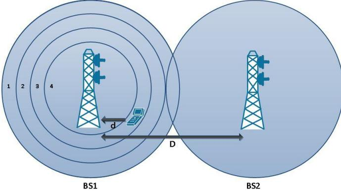
Figure 1. Network model for SNR calculations.
