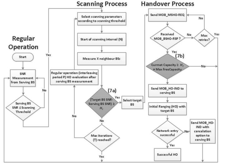
Figure 2. Flow chart of the proposed handover algorithm [12].
