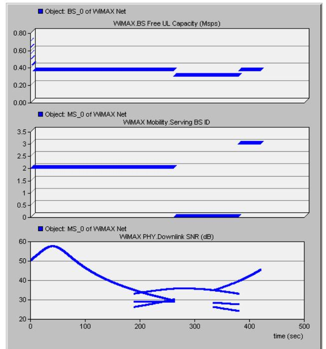
Figure 10. BS\_0 free upload capacity (top), serving BS ID for MS\_0 (middle), and downlink SNRs for MS\_0 (bottom).
