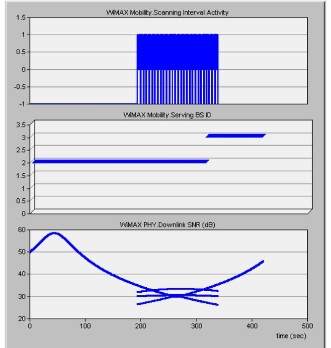
Figure 6. Scanning interval (top), serving BS ID (middle), and downlink SNRs (bottom) for MS $_0$ .
