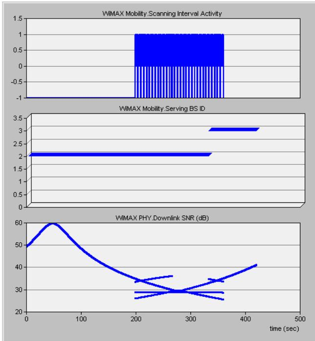
Figure 8. Scanning interval (top), serving BS ID (middle), and downlink SNRs (bottom) for MS\_0.
