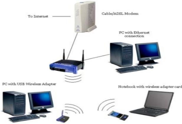
Figure 3: WiFi client/station connection [5].
