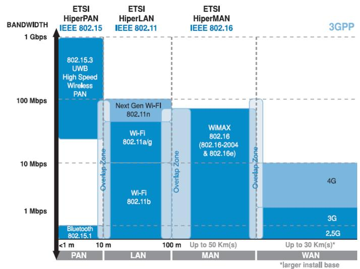
Figure 1: Bandwidth and coverage of wireless technologies [2].
