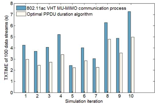
Fig. 4. Performance comparison of 10 simulations showing transmission times of 100 STAs.
