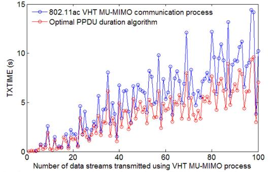
Fig. 3. Performance comparison of standard VHT MU-MIMO system and the proposed optimal PPDU duration algorithm.
