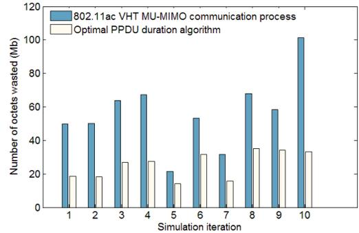
Fig. 5. Performance comparison of 10 simulations showing wasted portions of space-time streams of 100 STAs.
