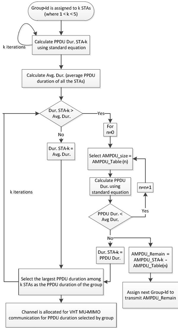
Fig. 2. Optimal PPDU duration algorithm: calculation of the TXTIME in VHT MU-MIMO systems.
