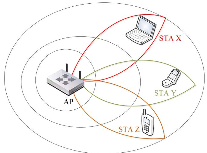
Fig. 1. VHT MU-MIMO system with three STAs.
