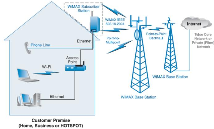
Figure 6. WiMAX client station connection.
