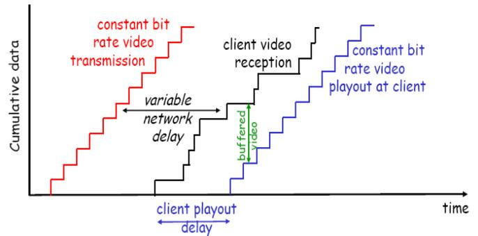
Figure 3. Buffering required at a video client.
