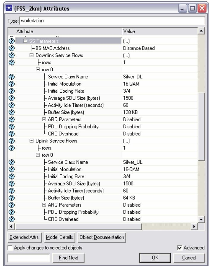
Figure 13. FSS service flow modulation and coding rates.
