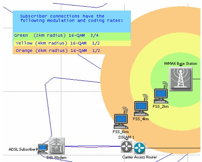
Figure 9. Simulation model of the video client subnet.
