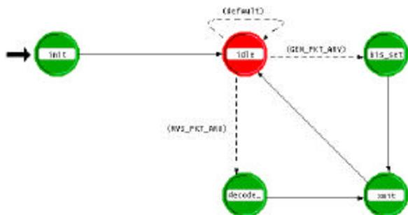
Fig. 6. FSM of the mdbs\_mac process model inside the MDBS node model. This process model implements the MAC protocol for the MDBS.
