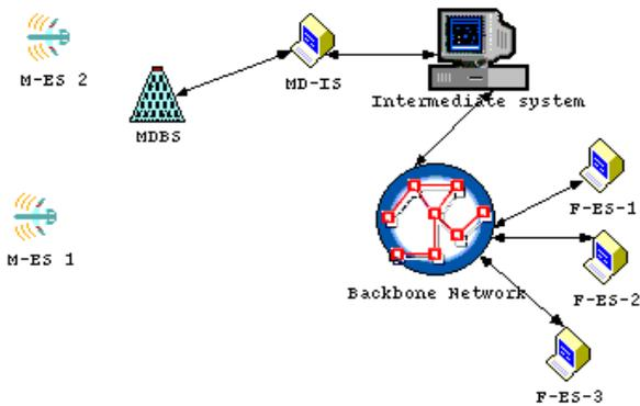
Fig. 1. Topology of a CDPD network. Each mobile end station (M-ES) is connected to the backbone network through the mobile data base station (MDBS). Fixed end systems (F-ES) are connected to the wired backbone network.
