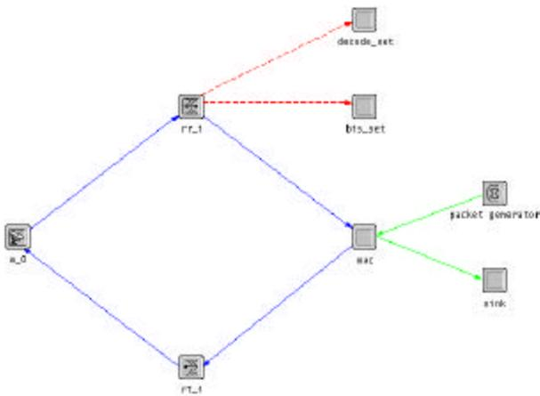
Fig. 4. Mobile data base station (MDBS) node model. This is the interface between the wireless and the wired sections of a CDPD network.
