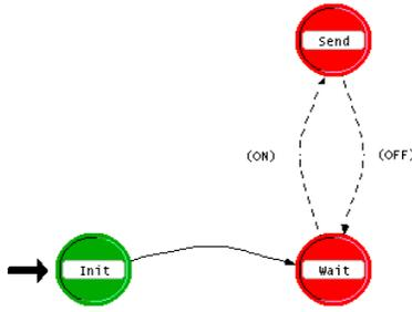
Fig. 8. ON/OFF OPNET traffic source model used inside M-ES. This process model generates packets in “send” state and rests in the “wait” state. Adjustment of the traffic burstiness is achieved by modifying the duration of these two states (ON/OFF time).
