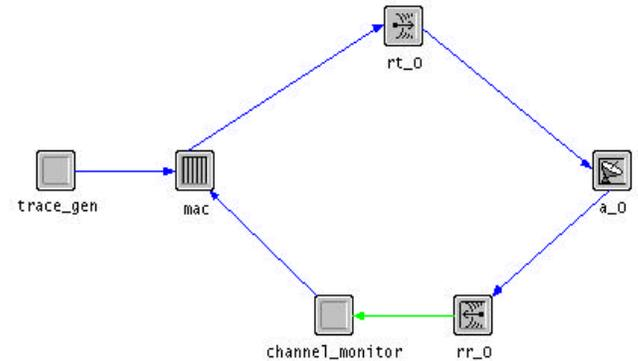
Fig. 3. Node model for mobile end system (M-ES). The radio transmitter is operating at a center frequency of 825 MHz. The radio receiver is operating at a center frequency of 870 MHz. Both have bandwidth of 30 kHz.
