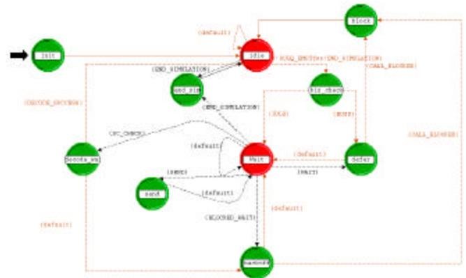
Fig. 5. FSM of `cdpd_mes_mac` process model. It performs media access control for the CDPD MAC interface in an M-ES.
