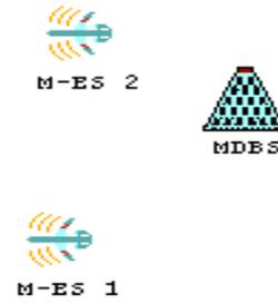
Fig. 2. Network model for the air interface. The two M-ES's send packets to the MDBS via the reverse channel at a center frequency of 825 MHz. They receive packets from the MDBS via the forward channel at a center frequency of 870 MHz.
