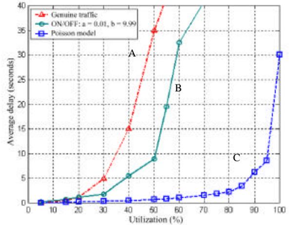
Fig. 9. Average delay vs. utilization plots for genuine traffic trace (graph A), traffic generated by ON/OFF model (graph B), and traffic generated by the traditional Poisson model (graph C).
