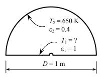
**15-89** A hemisphere with specified base and dome temperatures and heat transfer rate is considered. The emissivity of the dome is to be determined.
