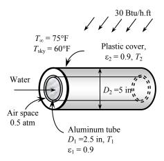
**Analysis** We have a horizontal cylindrical enclosure filled with air at 0.5 atm pressure. The problem involves heat transfer from the aluminum tube to the glass cover and from the outer surface of the glass cover to the surrounding ambient air. When steady operation is reached, these two heat transfer rates must equal the rate of heat gain. That is,
