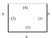
**15-54** The view factors from the base of a cube to each of the other five surfaces are to be determined.
