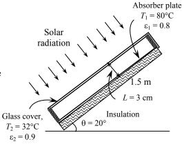
**Analysis** For  $\theta = 0^{\circ}$ , we have horizontal rectangular enclosure. The characteristic length in this case is the distance between the two glasses  $L_c = L = 0.03$  m Then,
