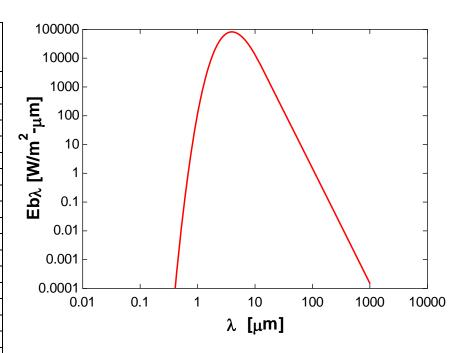
**15-23** The temperature of the filament of an incandescent light bulb is given. The fraction of visible radiation emitted by the filament and the wavelength at which the emission peaks are to be determined. *Assumptions* The filament behaves as a black body.
