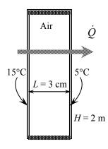
Analysis The characteristic length in this case is the distance between the glasses,  $L_c = L = 0.03$  m
