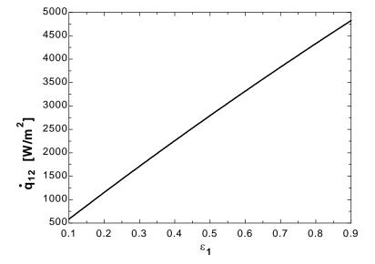
**15-71** The base, top, and side surfaces of a furnace of cylindrical shape are black, and are maintained at uniform temperatures. The net rate of radiation heat transfer to or from the top surface is to be determined.
