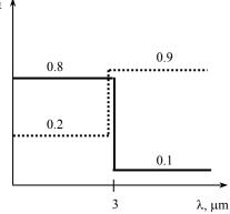
**15-38** The variation of emissivity of a surface with wavelength is given. The average emissivity and absorptivity of the surface are to be determined for two temperatures.
