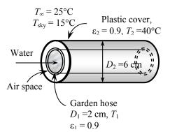
$$Ra = \frac{g\beta(T_s - T_\infty)D_2^3}{v^2} \Pr = \frac{(9.81 \text{ m/s}^2)(0.003273 \text{ K}^{-1})(40 - 25)\text{K}(0.06 \text{ m})^3}{(1.632 \times 10^{-5} \text{ m}^2/\text{s})^2} (0.7275) = 2.842 \times 10^5$$
