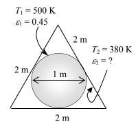
(b) The net rate of radiation heat transfer can be expressed for this two-surface enclosure to yield the emissivity of the enclosure:
