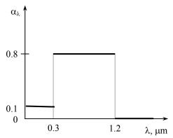
**15-95** The spectral transmissivity of a glass cover used in a solar collector is given. Solar radiation is incident on the collector. The solar flux incident on the absorber plate, the transmissivity of the glass cover for radiation emitted by the absorber plate, and the rate of heat transfer to the cooling water are to be determined.
