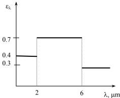
**15-34** The variation of reflectivity of a surface with wavelength is given. The average reflectivity, emissivity, and absorptivity of the surface are to be determined for two source temperatures.
