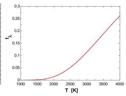
15-25 An incandescent light bulb emits 15% of its energy at wavelengths shorter than 0.8  $\mu$ m. The temperature of the filament is to be determined.
