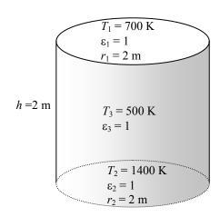
The view factor from the base to the top surface of the cylinder is  $F_{12} = 0.38$  (From Figure 15-7). The view factor from the base to the side surfaces is determined by applying the summation rule to be
