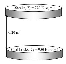
$$F_{12} = F_{ij} = \frac{1}{2} \left\{ S - \left[ S^2 - 4 \left( \frac{R_j}{R_i} \right)^2 \right]^{1/2} \right\} = \frac{1}{2} \left\{ 3.7778 - \left[ 3.7778^2 - 4 \left( \frac{0.75}{0.75} \right)^2 \right]^{1/2} \right\} = 0.2864$$
