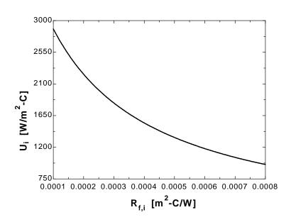
**16-24** Refrigerant-134a is cooled by water in a double-pipe heat exchanger. The overall heat transfer coefficient is to be determined.
