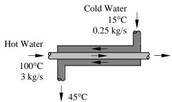
**16-105 EES** Prob. 16-104 is reconsidered. The effects of the inlet temperature of hot water and the heat transfer coefficient on the rate of heat transfer and the surface area are to be investigated.
