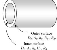
**16-22** Water is flowing through the tubes in a boiler. The overall heat transfer coefficient of this boiler based on the inner surface area is to be determined.
