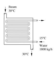
**16-110 EES** Prob. 16-109 is reconsidered. The effects of the condensing steam temperature and the tube diameter on the rate of heat transfer and the rate of condensation of steam are to be investigated.
