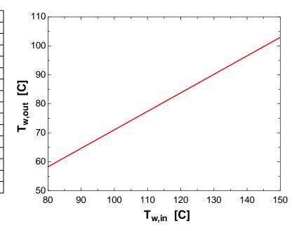
**16-98** Water is heated by hot air in a heat exchanger. The mass flow rates and the inlet temperatures are given. The heat transfer surface area of the heat exchanger on the water side is to be determined.
