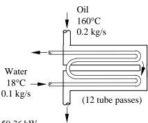
**16-95E** Inlet and outlet temperatures of the hot and cold fluids in a double-pipe heat exchanger are given. It is to be determined the fluid, which has the smaller heat capacity rate and the effectiveness of the heat exchanger.
