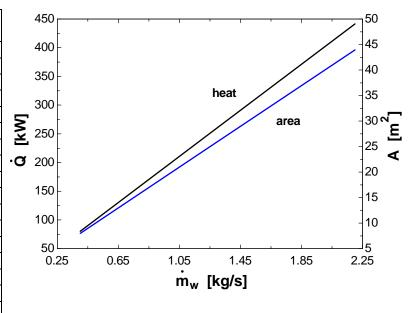
**16-66E** Steam is condensed by cooling water in a condenser. The rate of heat transfer, the rate of condensation of steam, and the mass flow rate of cold water are to be determined.
