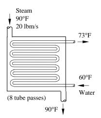
**16-67E EES** Prob. 16-66E is reconsidered. The effect of the condensing steam temperature on the rate of heat transfer, the rate of condensation of steam, and the mass flow rate of cold water is to be investigated. *Analysis* The problem is solved using EES, and the solution is given below.
