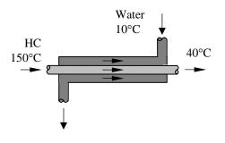
**16-45** Oil is heated by water in a 1-shell pass and 6-tube passes heat exchanger. The rate of heat transfer and the heat transfer surface area are to be determined.
