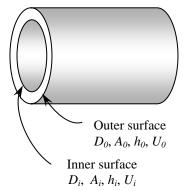
**16-126** Water is heated by hot oil in a multi-pass shell-and-tube heat exchanger. The rate of heat transfer and the heat transfer surface area on the outer side of the tube are to be determined.
