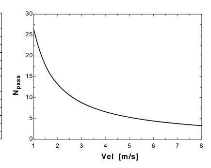
**16-118** Cooling water is used to condense the steam in a power plant. The total length of the tubes required in the condenser is to be determined and a suitable HX type is to be proposed.
