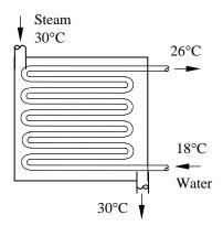
**16-119** Cold water is heated by hot water in a heat exchanger. The net rate of heat transfer and the heat transfer surface area of the heat exchanger are to be determined.
