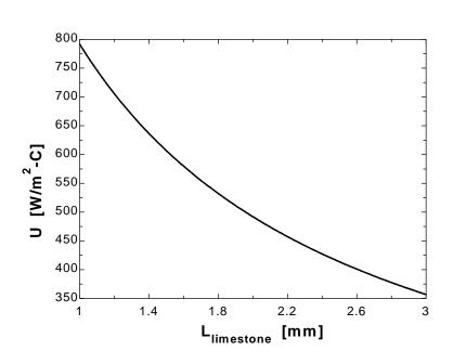
**16-27E** Water is cooled by air in a cross-flow heat exchanger. The overall heat transfer coefficient is to be determined.
