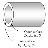
**16-125** Hot oil is cooled by water in a multi-pass shell-and-tube heat exchanger. The overall heat transfer coefficient based on the inner surface is to be determined.
