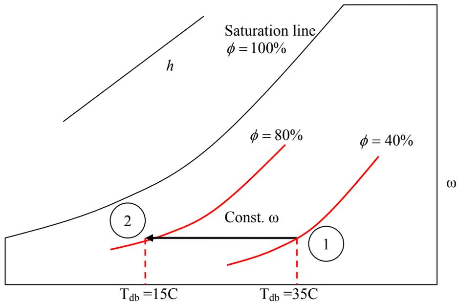
Fig.4: A simple cooling process.
