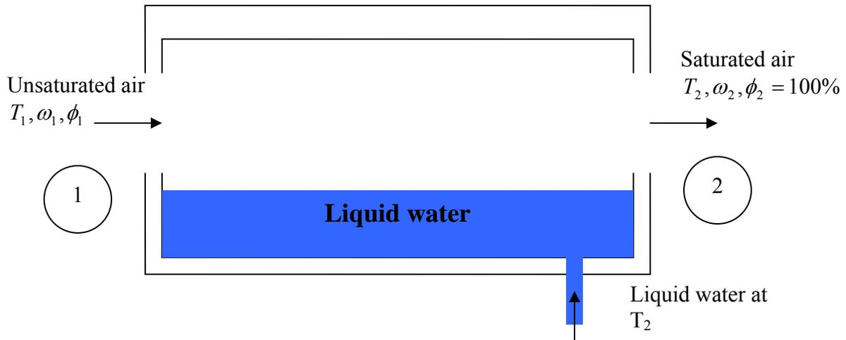
Fig. 1: Schematic of an air saturator.
