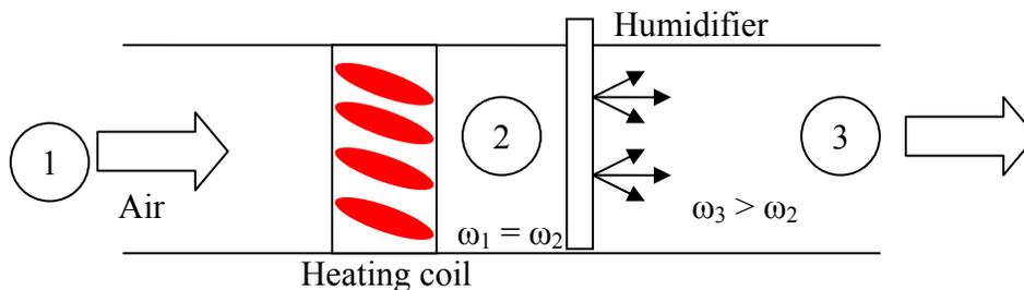
Fig. 5: Heating with humidification.
