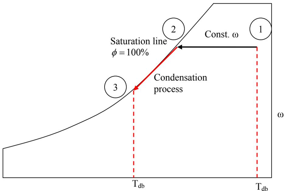
Fig. 7: Cooling with dehumidification.
