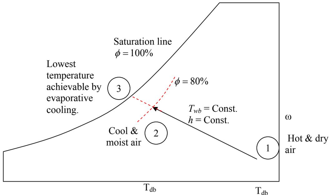
Fig. 8: Evaporative cooling.
