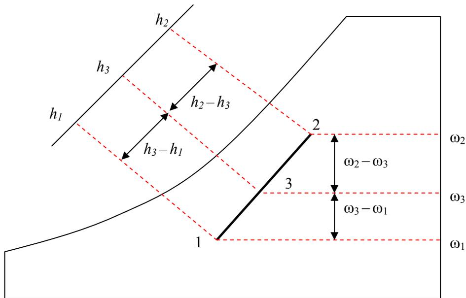
Fig. 9: Adiabatic mixing of two streams.
