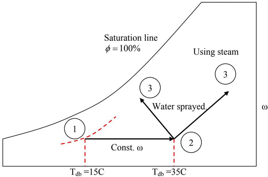
Fig. 6: Heating with humidification, using water spray or steam.
