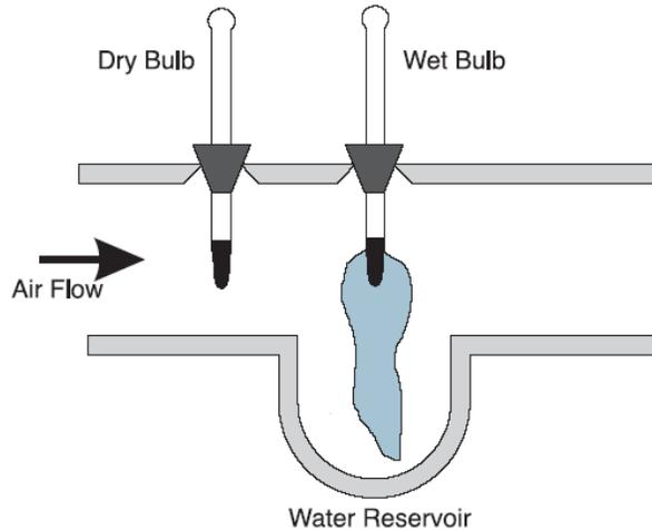
Fig.2: Dry bulb and wet bulb temperature.
