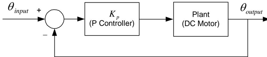
**Figure 2.9 Closed loop system with a proportional controller**
