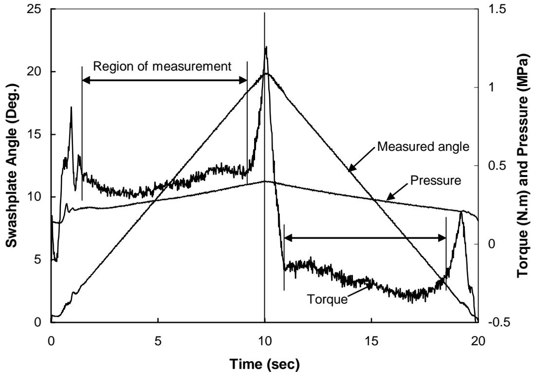
**Figure B.5 Frictional torque measurement design**
