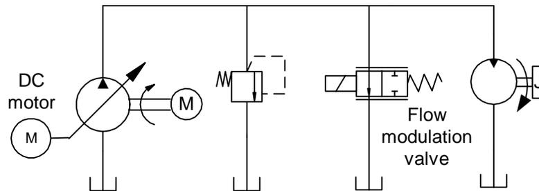
**Figure 2.1 Pump-controlled system with the bypass flow control**
