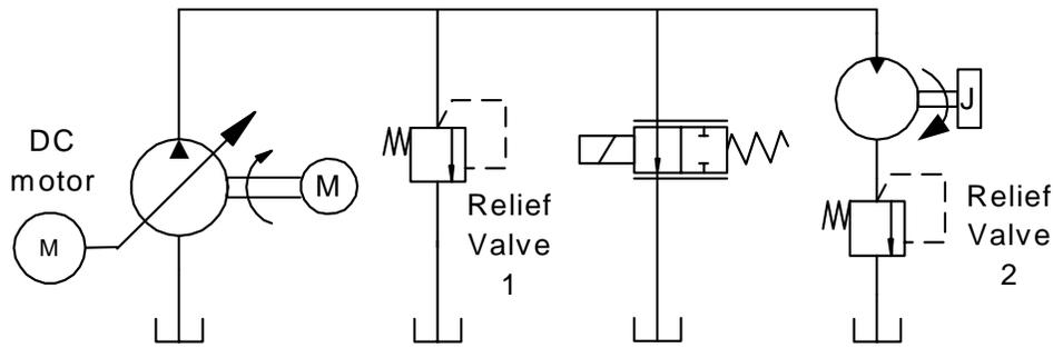
**Figure 2.5 Pump-controlled system with bypass flow control**
