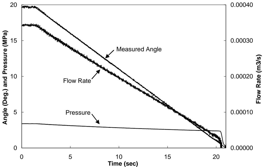
**Figure 3.6 Measured steady state performance of the DC motor controlled pump
