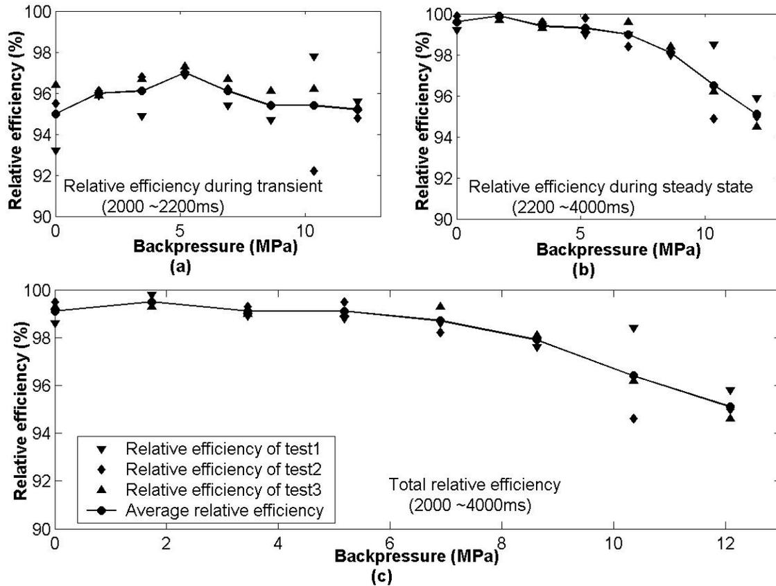
**Figure 5.8 Relative efficiency of the bypass control system**
