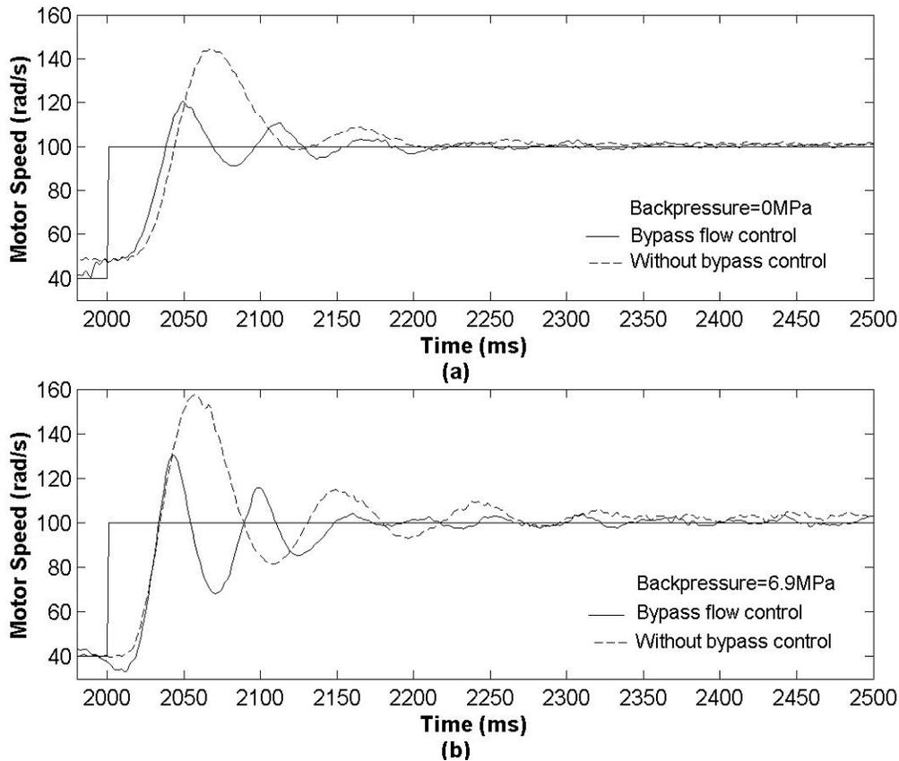
**Figure 5.13 Dynamic responses of the motor with 2 redesigned controllers
