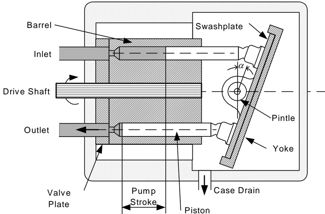
**Figure 2.2 Schematic of variable displacement piston pump**
