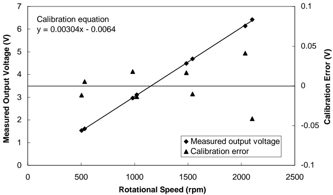
Figure A.6 Calibration of tachometer
