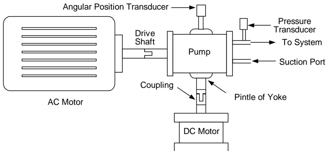
**Figure 2.3 Direct swashplate control with a DC motor**
