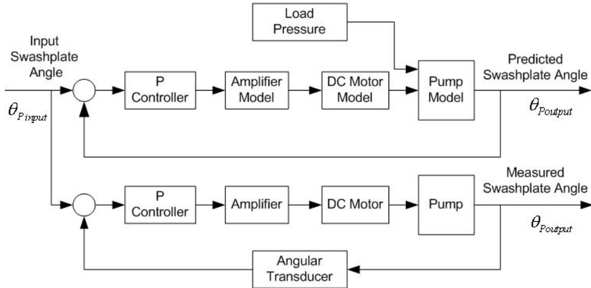
**Figure 3.1 Block diagram of pump performance test**
