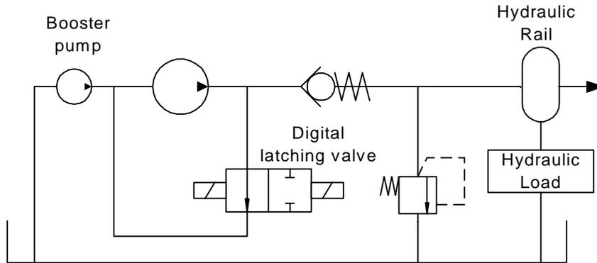
**Figure 1.2 Variable flow supply using latching valve [Mansouri, 2001]**
