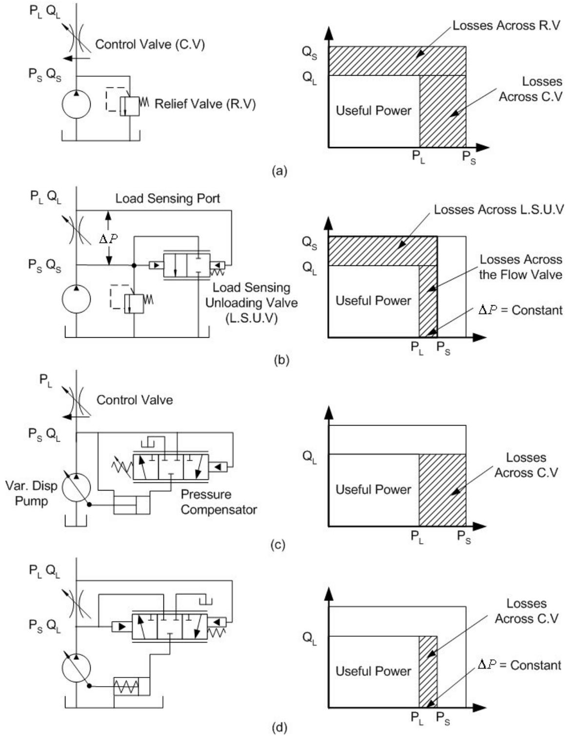
**Figure 1.1 Power losses of valve-controlled systems**
