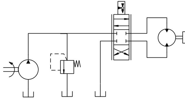
**Figure 1.13 Valve controlled motor system with a constant flow supply**
