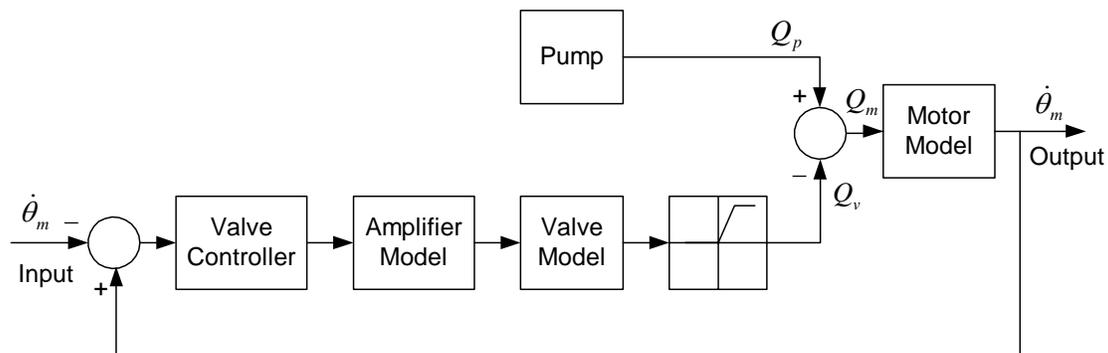
**Figure 4.5 Block diagram of bypass flow control system**
