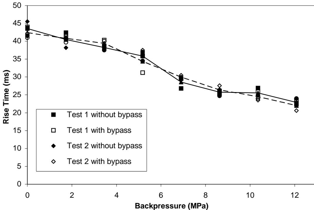
**Figure 5.5 Rise time of the motor rotational speed**
