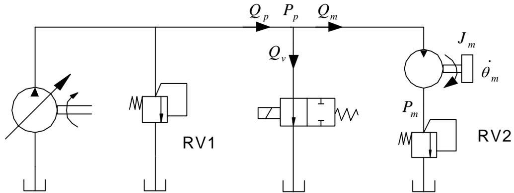
**Figure D.4 Schematic diagram of the hydraulic circuit**
