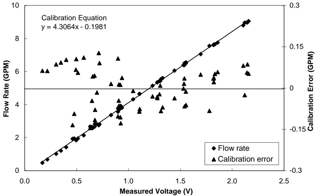
**Figure A.7 Calibration of flow meter**
