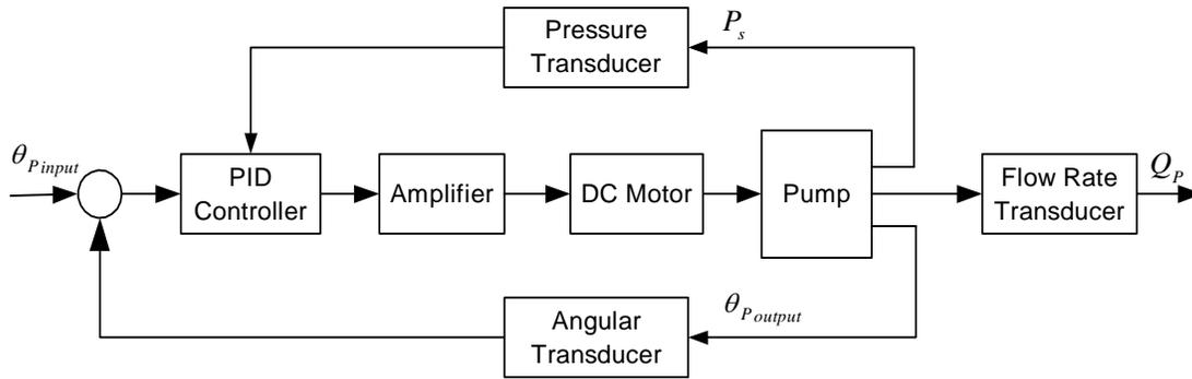
**Figure 3.5 Block diagram of pump performance test**
