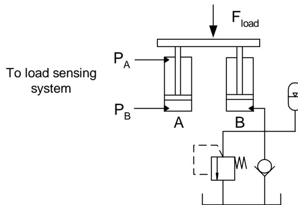
**Figure 1.11 Schematic of an energy reutilization system**
