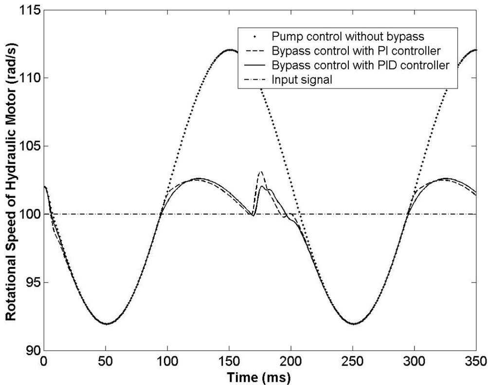
**Figure 4.10 Comparison of resetable PI and PID controllers**
