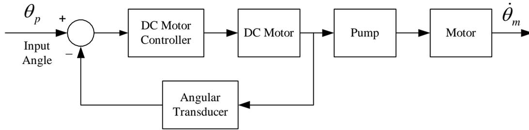
**Figure 2.6 Block diagram of DC motor control**
