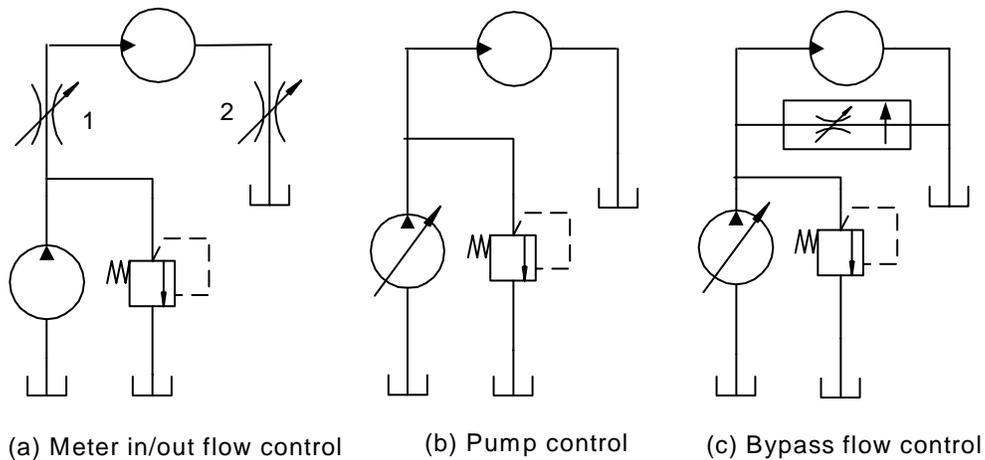
**Figure 2.4 Schematic of valve and pump controlled systems**
