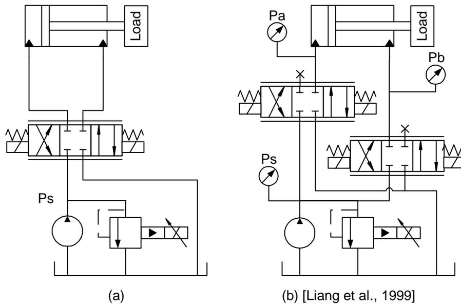
**Figure 1.3 Systems with meter-in and meter-out control**
