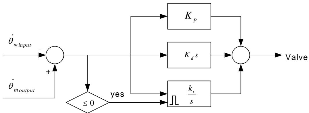
**Figure 4.9 Schematic of a “resetable” PID controller**
