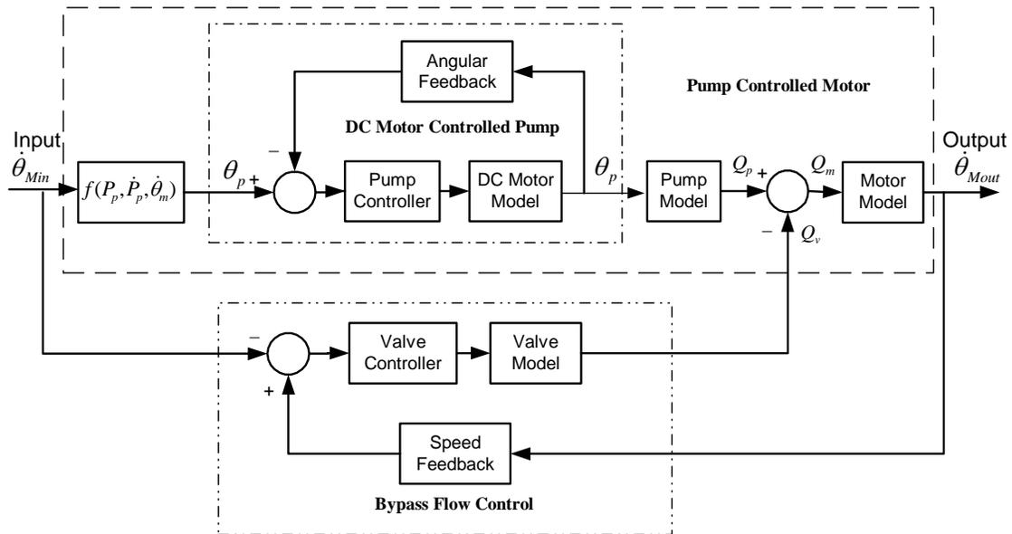
**Figure 4.1** Block diagram of the complete hydraulic system
