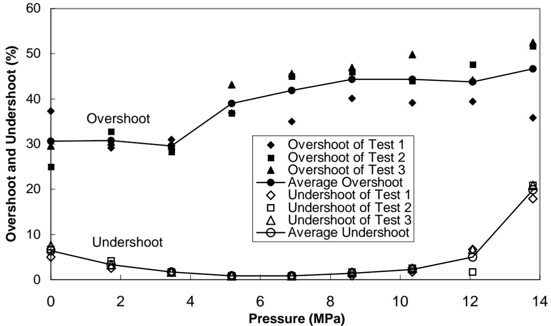
Figure 3.9 Overshoot and undershoot of pump swashplate angle
