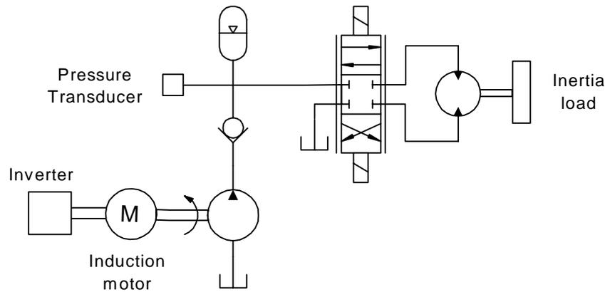
**Figure 1.9 Energy-saving power source with inverter-motor drive**
