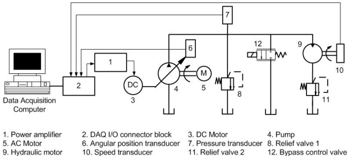
**Figure 2.7 Electrical interface and measurement system design**
