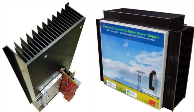
Figure 7: Sub-assembly consisting of a heat sink, heat pipes and rectifier (left); Full prototype (right)
