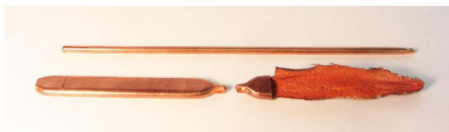
Figure 3: Circular heat pipe (top), flat heat pipe (bottom left) and cut flat heat pipe showing a sintered metal wick structure (bottom right)
