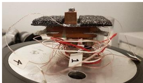
Fig. 2. Sorbent composite bolted to copper heat exchanger
