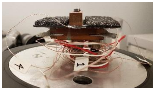
Fig. 2. Sorbent composite bolted to copper heat exchanger
