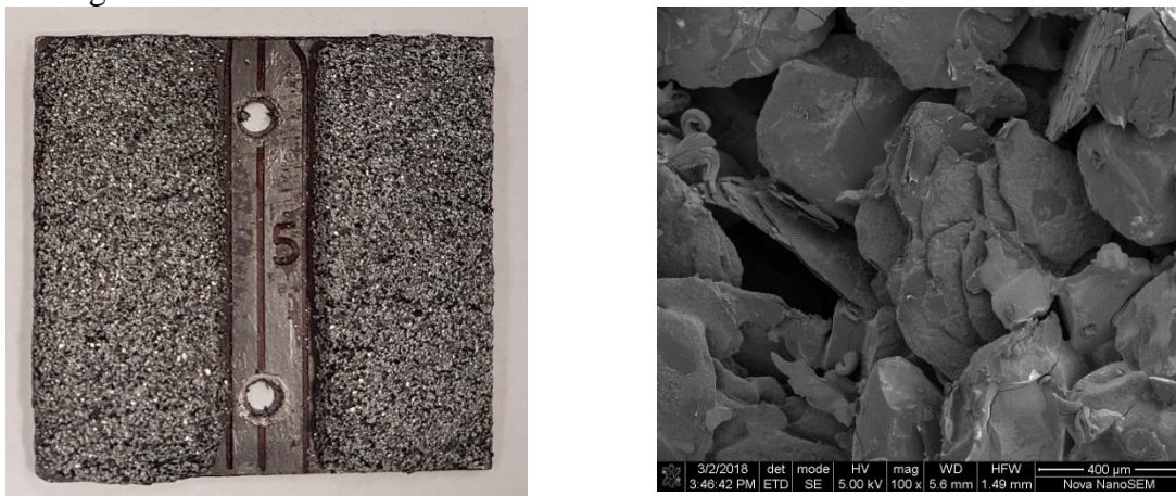
Fig. 1. The composite sorbent with 20 wt% graphite flake content coated on graphite sheets (left), SEM image (right)
