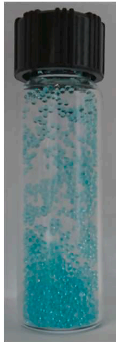
Fig. 12. Collected microcapsules (contain liquid desiccant: 60 wt% LiBr and 40 wt% deionized water).
