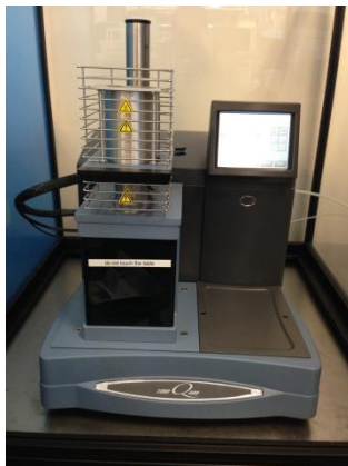
(a) (b) Figure 28. (a) TMA device, and (b) its schematic [104]
