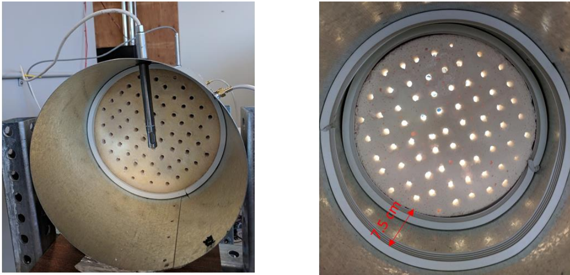
Figure 24 Sorbent discs placed in an 8.5” duct with 7.5 cm spacing and sealed by a rubber seal
