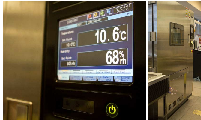
Figure 3.5: Environmental chamber (Platinous H-series, ESPEC, USA) used to simulate different environmental conditions.
