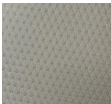
Figure 2.8 The patterned surface of 150μm-thick filter PTFE substrate
