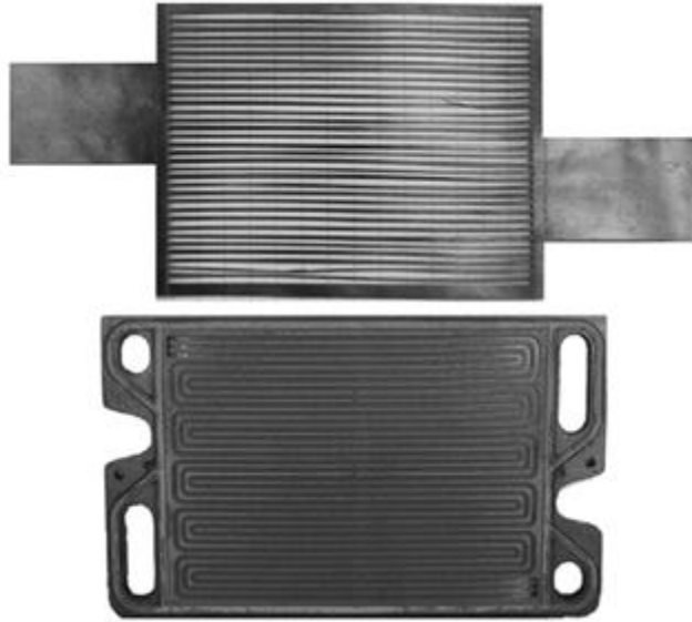
Figure 1-5: Picture of the flow channel plate and the shaped pyrolytic graphite sheets [30].
