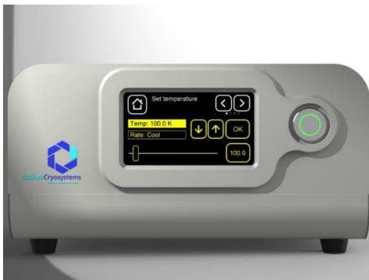
Figure 7: Touch screen (shown above in Command screen) and illuminated Start/Stop Button
