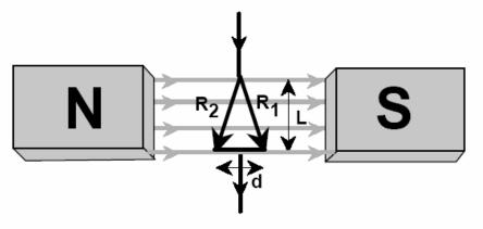
2(5/20 marks). What is the peak emf produced by a 50 turn square coil (of side l=10.0cm, as shown in the diagram below) rotating on an axis with a frequency of 30.0Hz in a uniform magnetic field of 0.750T perpendicular to the coil's axis of rotation?
